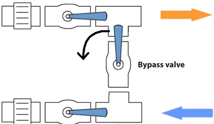
*First open all the valves to simplify adjustment of the bypass.*
