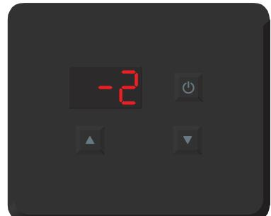
Change the set value using the arrow keys. The current sensor values can not be changed.
