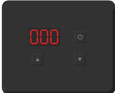
Once the up and down arrow keys have been pressed for ten second, the code 000 is shown.
