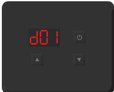
Press the up and down arrow for a few seconds to enter the selected category. Select the preferred parameter using the arrow keys.
