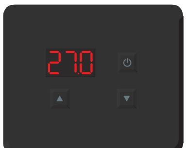
Revert to showing the current inlet temperature by pressing the On/Off button again.
