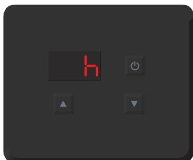
*Once the up and down arrow keys have been pressed for one second, the current operating mode is shown.*
