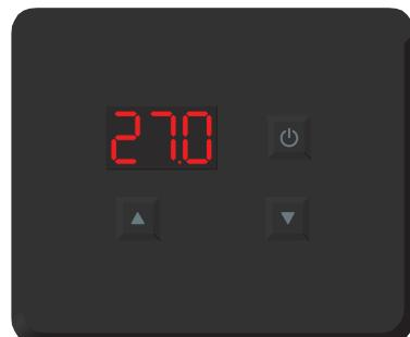
The display shows the incoming water temperature when the pool heat pump is running.
