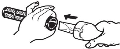
Cap Assembly and shake out the debris.
