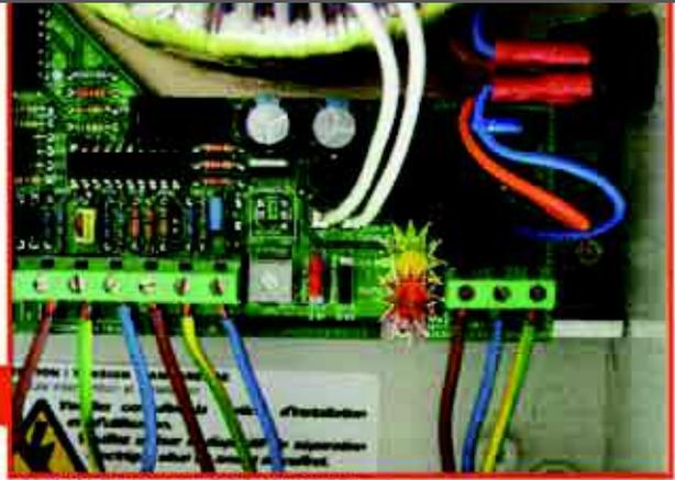
The red and yellow light-emitting diodes flash. If not, check the electric connections.
