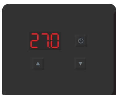
Revert to showing the current inlet temperature by pressing the On/Off button again.
