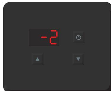
Change the set value using the arrow keys. The current sensor values can not be changed.
