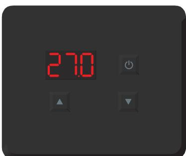
*Pressing one of the arrow keys displays the current preferred temperature in flashing mode.*
