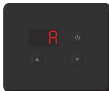
*Pressing the arrow keys repeatedly changes the operating mode. The set value is saved automatically after 5 seconds.*
