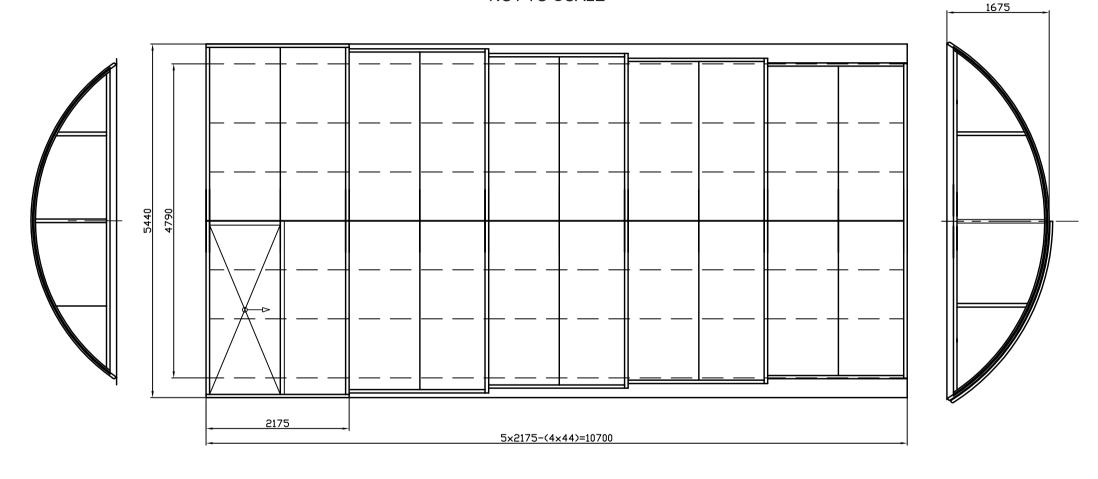
4790 mm - inner rail width 5440 mm - outer rail width
