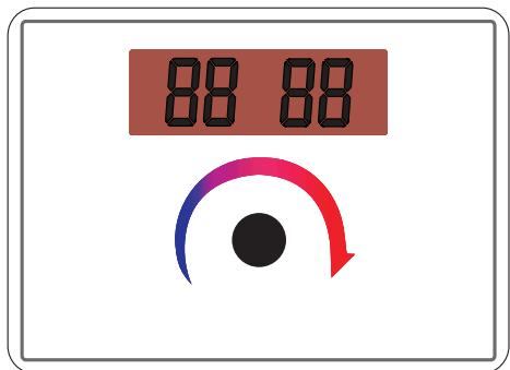
Press in the knob to start/stop the heat pump
