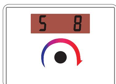
Parameter 5: Maximal defrosting time. (0 - 15 min)
