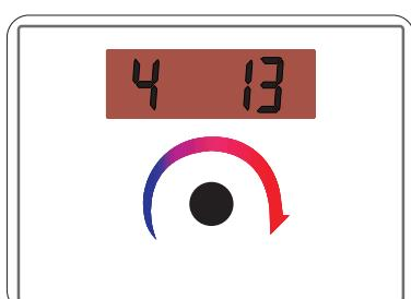
Parameter 4: Stop temperature for defrosting. (0 - 30 °C)
