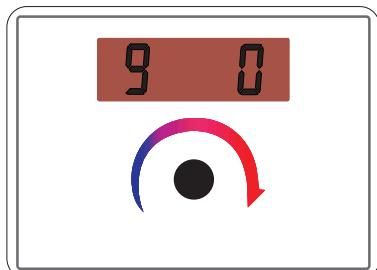
Parameter 9: External pump. (0 = Always running / 1 = Running at the same time as the compressor)
