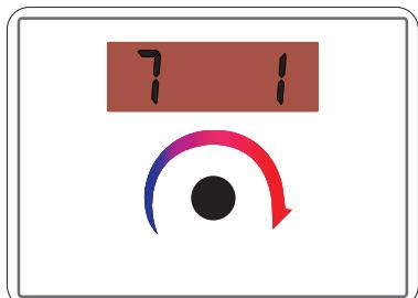
Parameter 7: Automatic restart on power failure. (0 = No / 1 = Yes)
