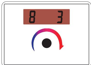
Parameter 8: (0 = Cooling mode / 1 = Heating mode or cooling mode / 2 = Not used / 3 = Heating mode)
